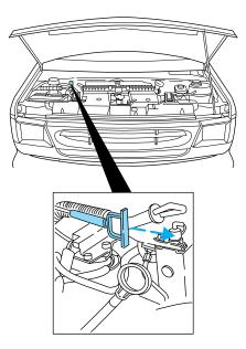
4. **On Econoline models,** open fuel filter drain valve by pulling on the release handle. Allow to drain for approximately 25 seconds or until clean fuel is observed. Close filter drain valve by resetting handle to original position.
